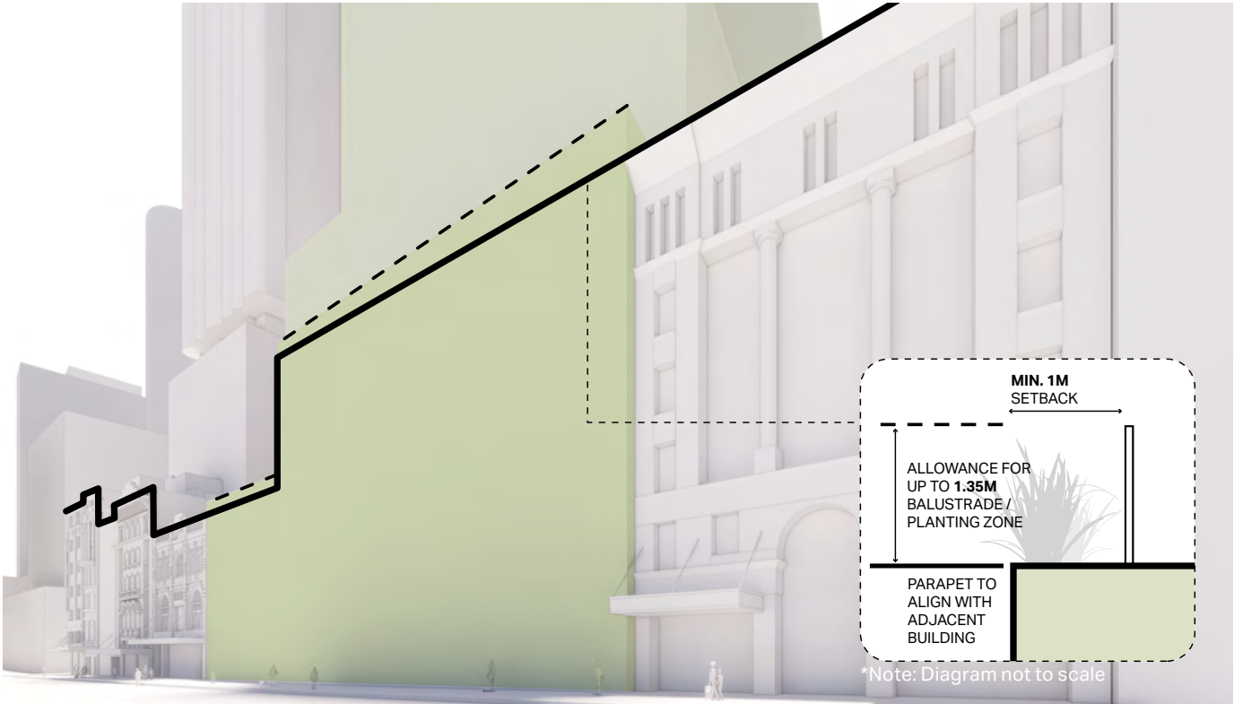
Proposed Envelope Close-up - Pitt Street, looking north.
